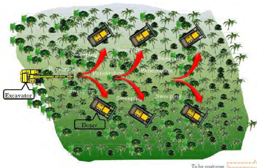
Figure 1: A drawing showing the proper way to clear a forest area
