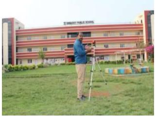
measurement was conducted as per IS:4954 as adopted by CPCB. Ambient noise level monitoring was carried out during December 2015.
