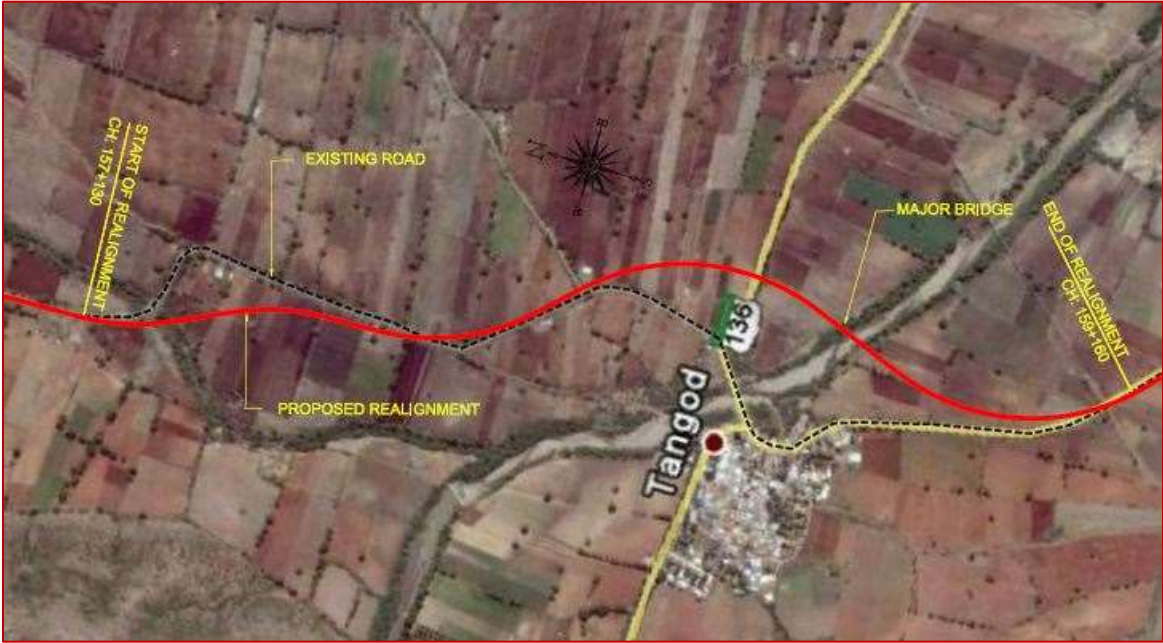
Figure 27: Proposed Realignment from Ch. 157+130 to Ch. 159+160 including Major Bridge at Ch. 158+591
