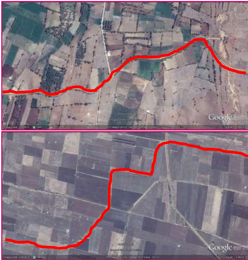
Figure 21: Project Road with Geometric deficiencies observed in majority sections
