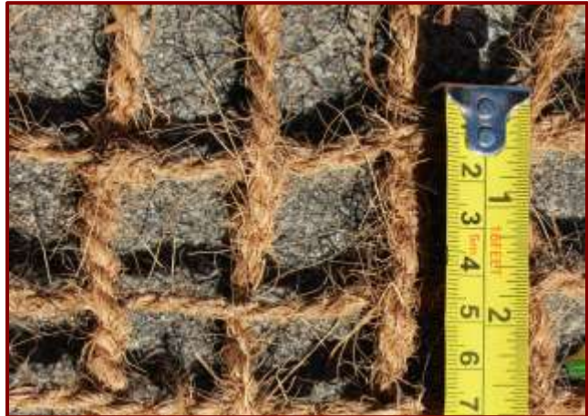
Coir geo-textiles specifications: Grade I- 400g/m 2
