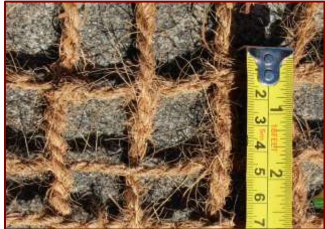
Coir geo-textiles specifications: Grade I- 400g/m 2
