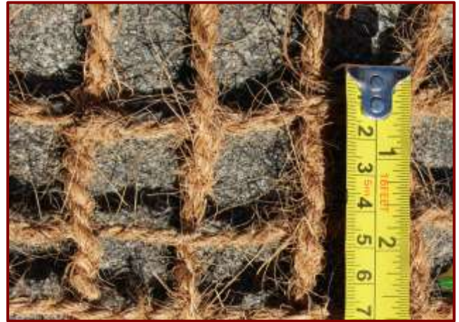
Coir geo-textiles specifications: Grade I- 400g/m 2
