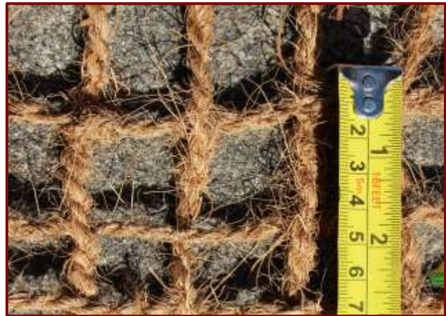
Coir geo-textiles specifications: Grade I- 400g/m 2
