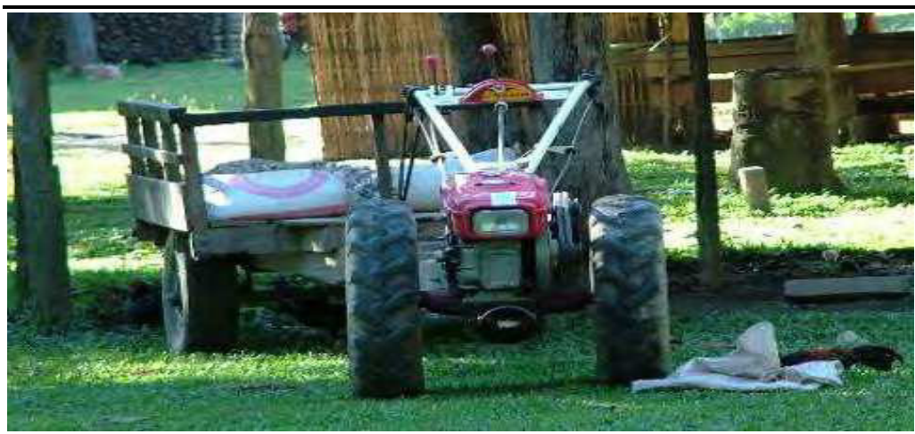
Figure 5.33 Two-Wheel Tractor Pulling a Cart
