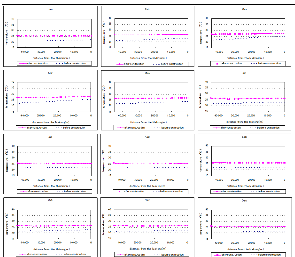
Figure 6.18 Comparison of Downstream Water Temperatures of NNP1
