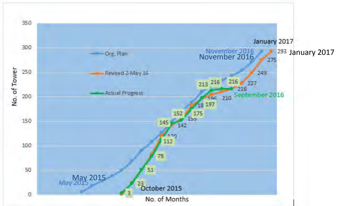
Figure 3-4: Cumulative Work Progress (Plan and Actual)
