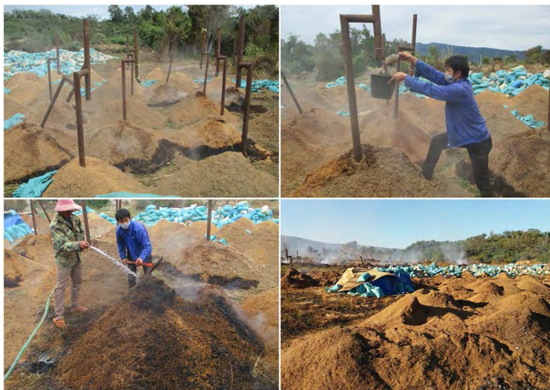
FIGURE 15-3 PREPARATION OF BIO-CHAR FROM RISK HUSK FOR USE AS SOIL IMPROVEMENT MATERIALS FOR PADDY RICE FIELDS BEING DEVELOPED FOR 2LR RESETTLERS (DECEMBER 2016)
