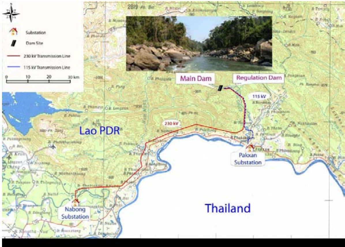
Figure 1-1 Alignment of the 230 kV and 115 kV transmission lines.
