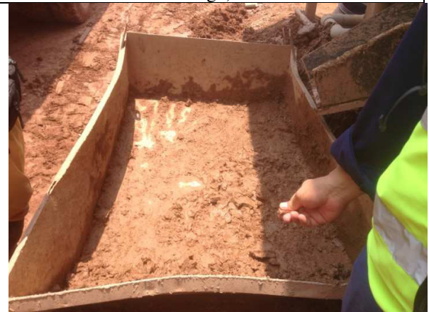
The sludge coming out from the plant (the “cake”)
