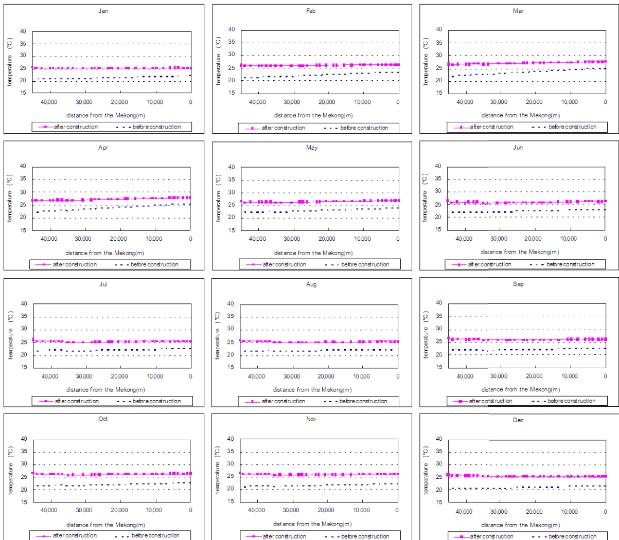
Figure 7-15 Comparison of downstream water temperatures of NNHP-1.
