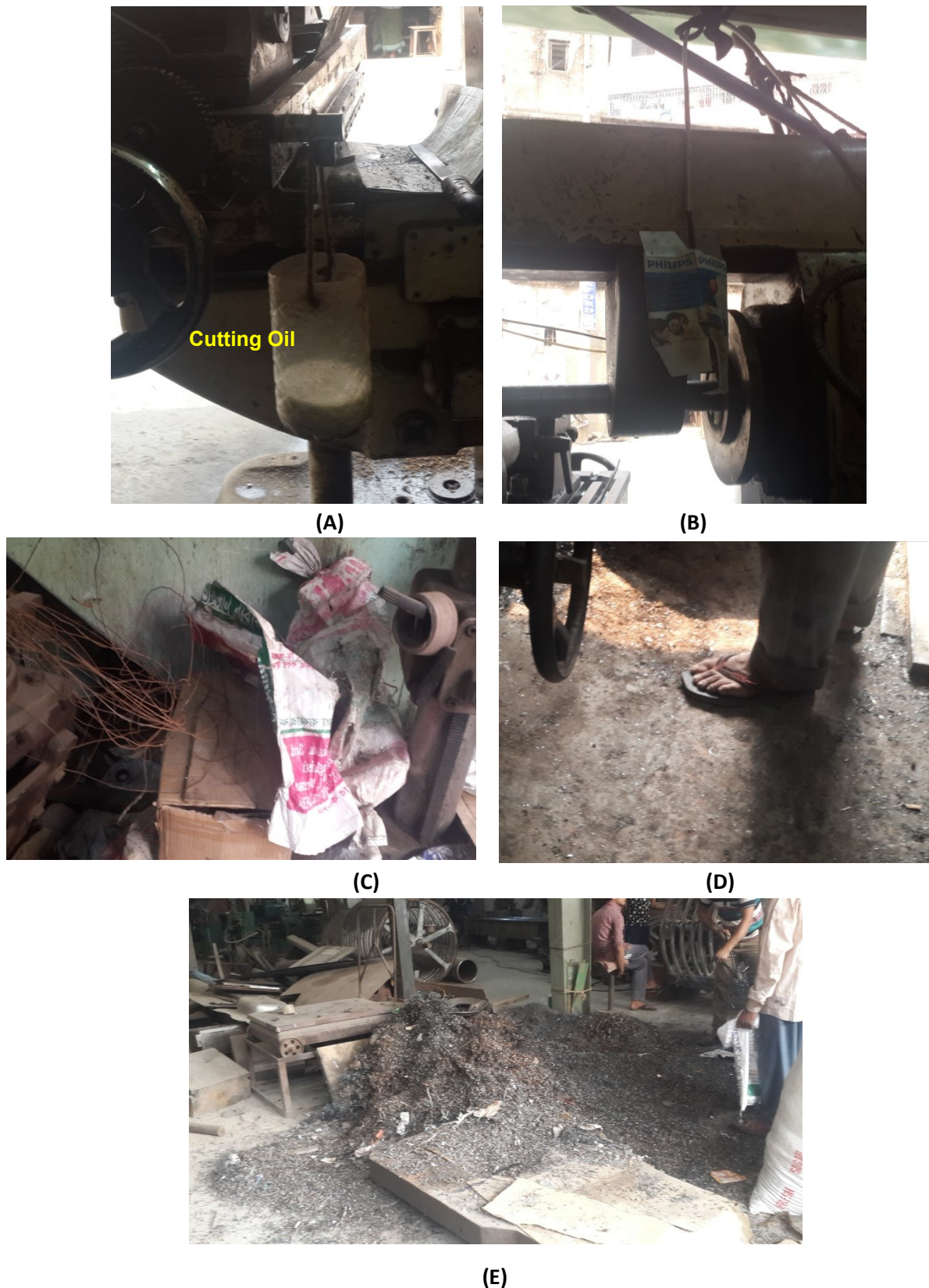
Figure 5.1: (A) Improper storage and handling of Cutting Oil; (B) Inadequate lighting and electrical connections can lead to accidents; (C) Lack of cleanliness reduces productivity; (D) Workers need to have protective footwear; (E) Improper waste management
