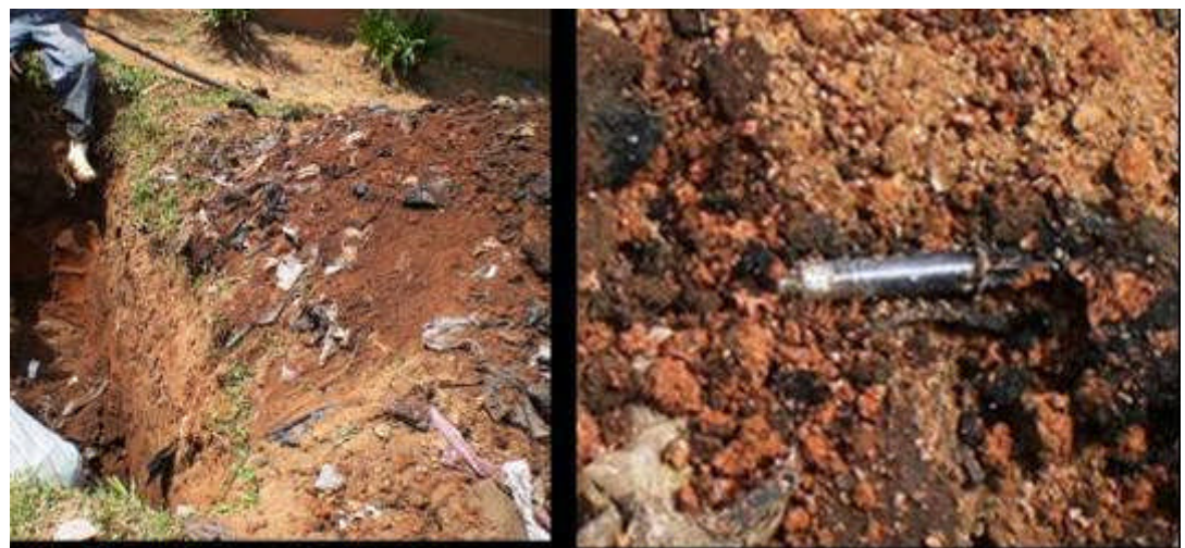
Figure 7-9, Excavation of deep buried sharps after 5 years (Tanzania, Tanga, 2009)
