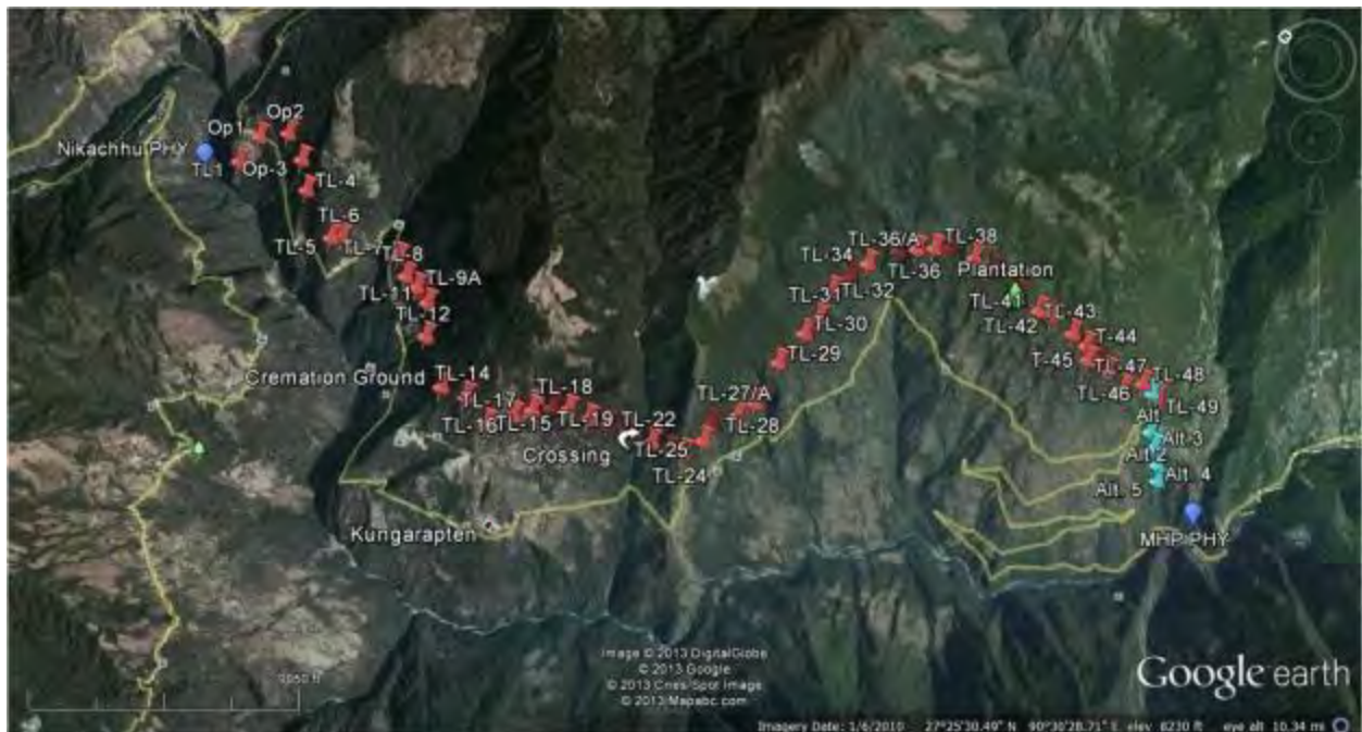
Figure 3.1: TL alignment showing the location of the towers
