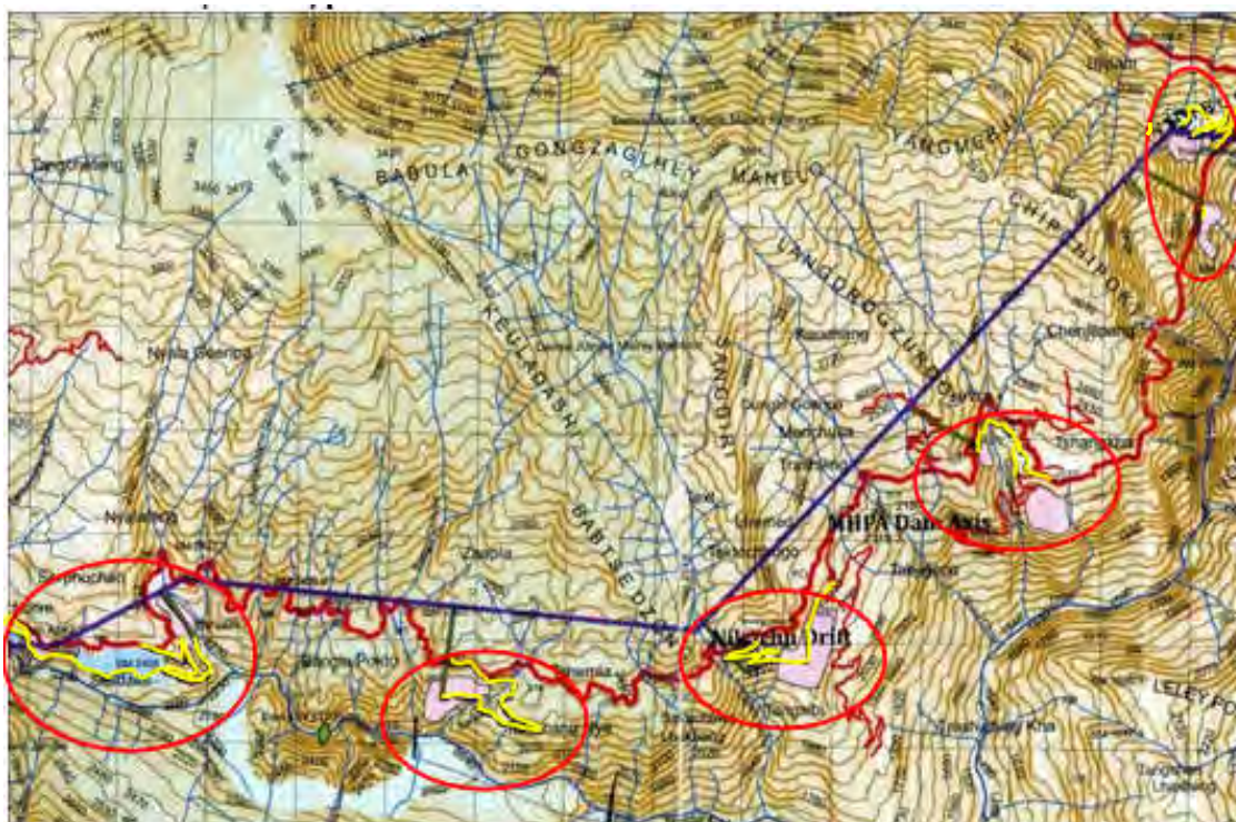
Figure 2-12: Locations of proposed access roads (in yellow), muck disposal areas (in pink), and colonies (in blue).
