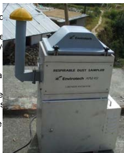
Figure 46 : High Volume Air Sampler
