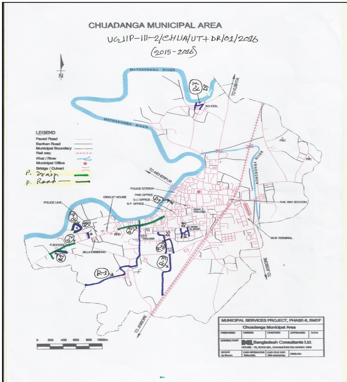
Figure 2: Proposed roads & drains sub-project in Pourashava under UGJIP –III
