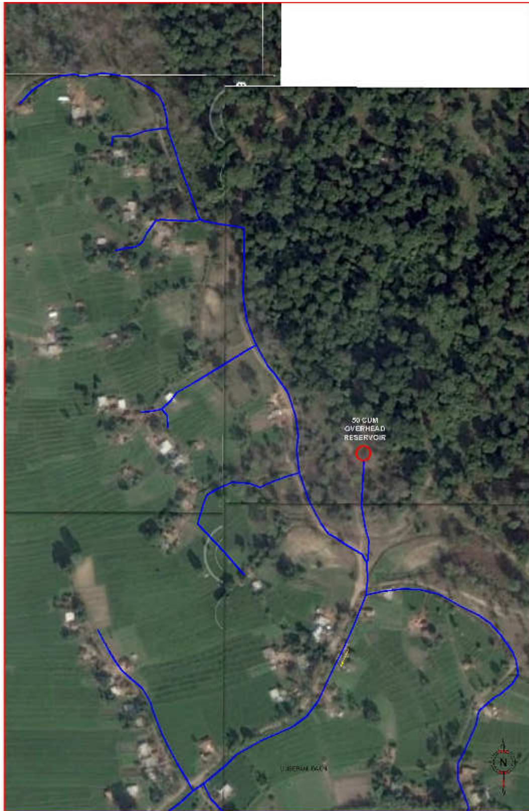
Google based map showing the location of proposed 50 Cum OHT, Tube Well (5.5 lps) and Treatment Plant (5.5 lps) for East sub-system (Musepani Sub-system).
