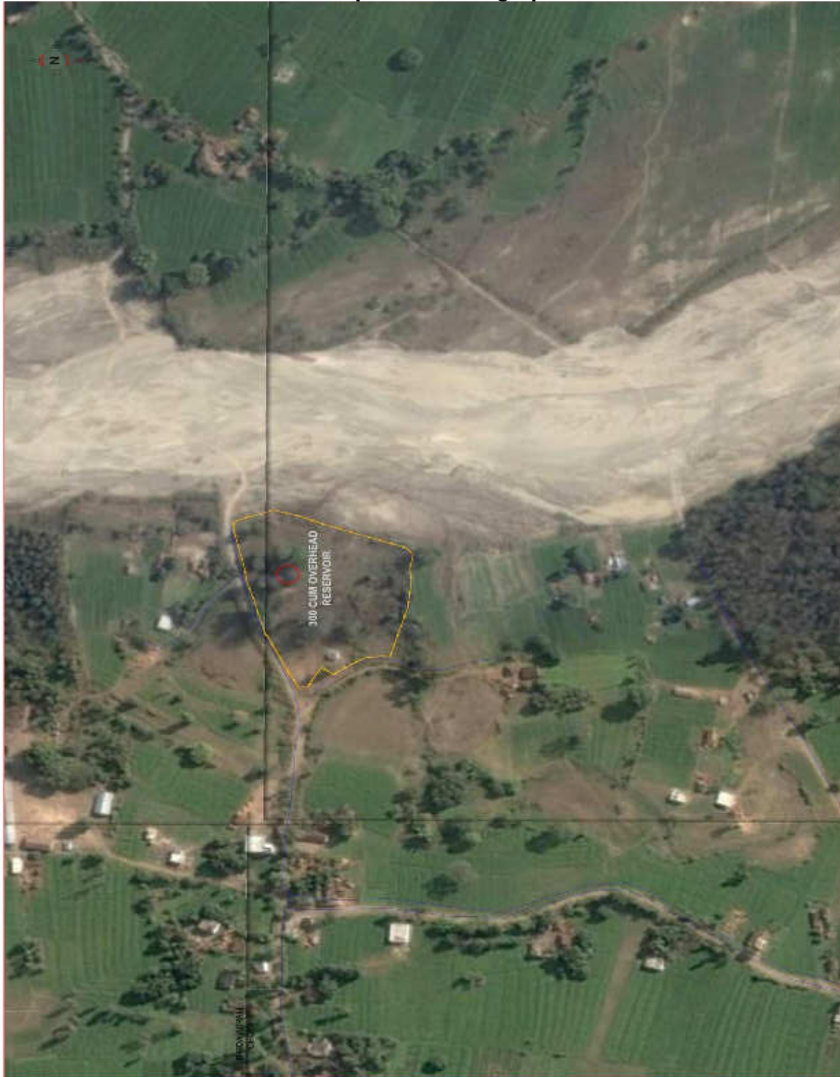
Google based map showing the location of proposed OHT (300 Cum), Tube well (32.42 lps) and Treatment Plant (32.42 lps) for South Sub-system. Office Building will also be located on the same site (within marked area).
