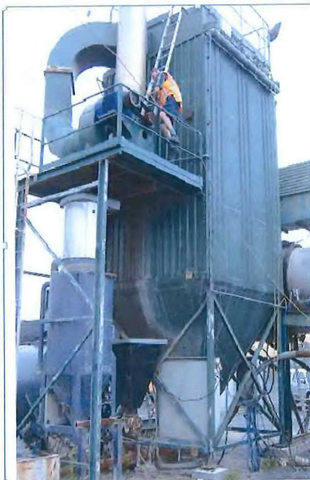
Figure 1 MacDow Drum Mix Plant – (left) Baghouse, Compressor, Fan stand. Baghouse in operation in 2009 at Taotaoroa Quarry / SWAPS Quarry – Waikato NZ.
