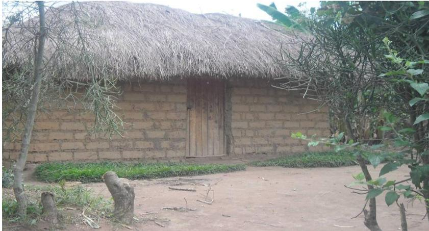
**Figure 2: Grass thatched hut in the areas of Soroti. The wall is made of unburnt bricks due to increasing lack of wood and economic status of the communities.**
