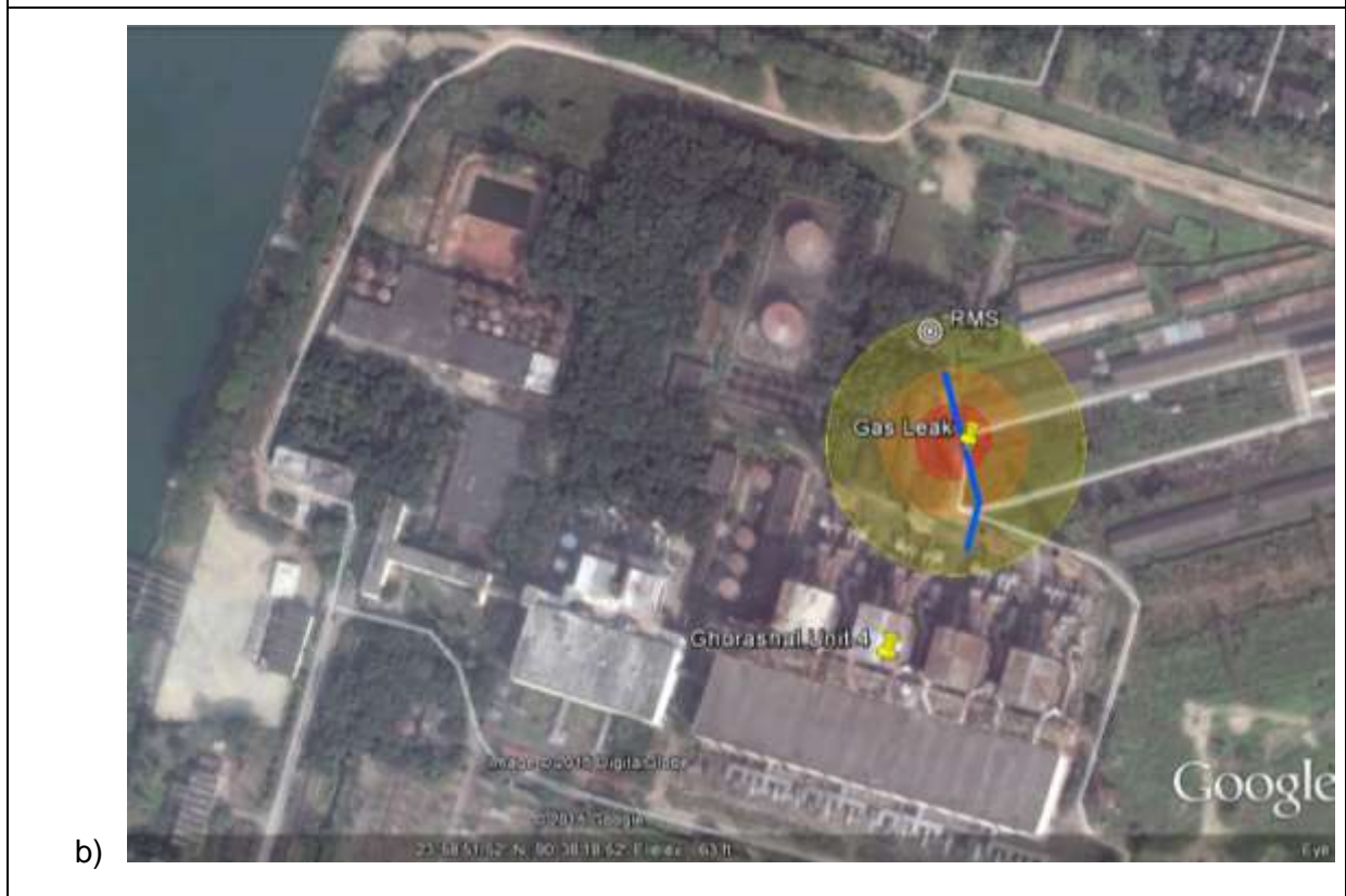
Figure 10-4: Threat Zone of Thermal Heat Radiation of a Jet Fire from gas leak
