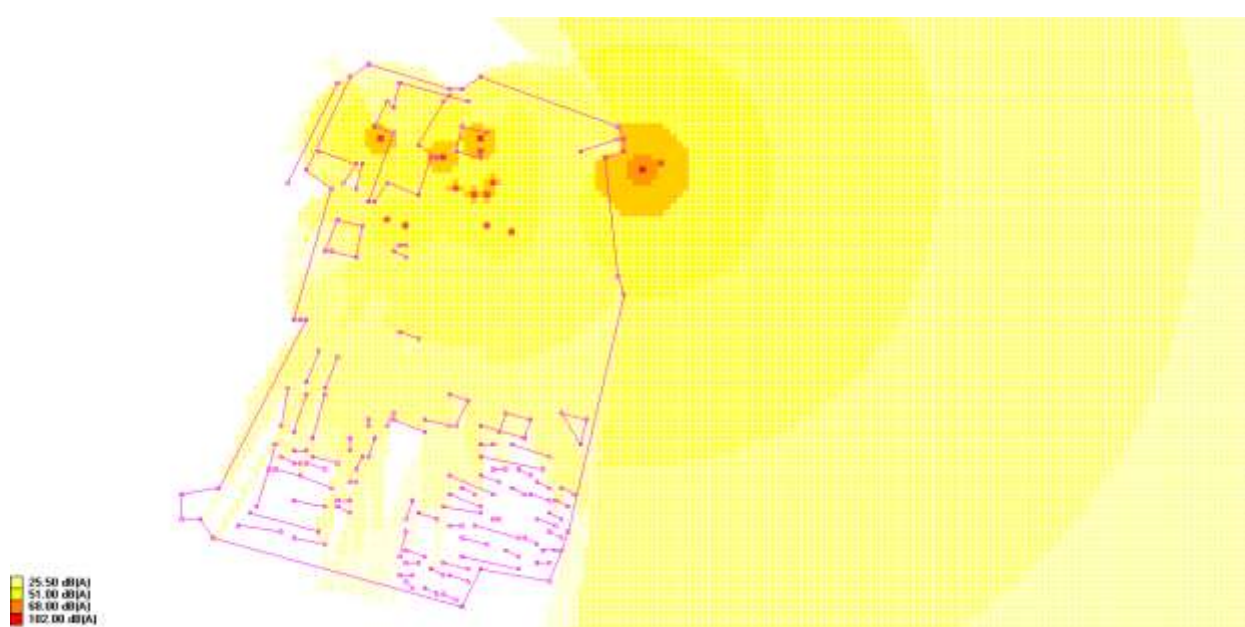
Figure 7-26: Simulation of Noise Propagation during Plant Operation in Cumulative Scenario
