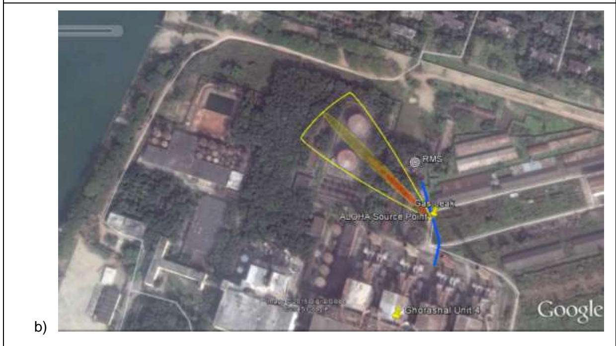
Figure 10-3: Threat Zone of Flammable Vapor Cloud resulted from a Gas Pipeline Leakage
