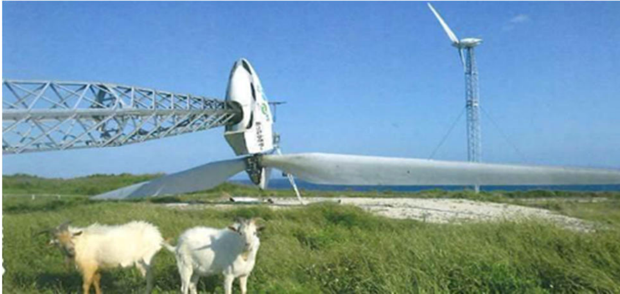
Figure 5.1: Example of Fold-down Turbine Design (1 turbine upright and 1 prone)
