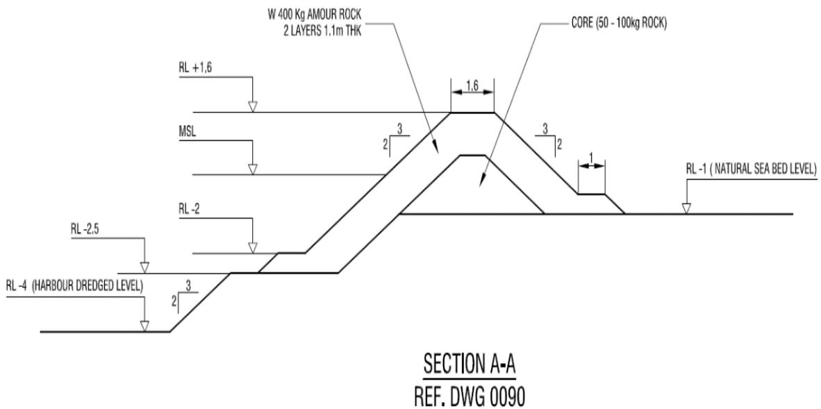
Figure 13: Breakwater – Section B
