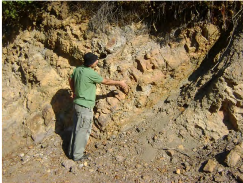
Figure 4.4: Altered and Jointed Chouf Sandstone and Eboulis.
