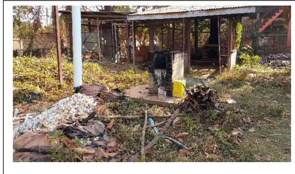
Storing and malfunction of incinerator – SothNikum RH
