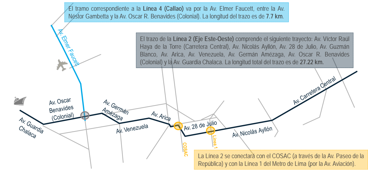
Figure 3: Selected Alignment for Metro Line 2 (and Line 4 Branch), Integration Points and Feeder Network with COSAC (Metropolitano BRT) and Metro Line 1 (Tren Electrico) (Source: Project Feasibility Study)
