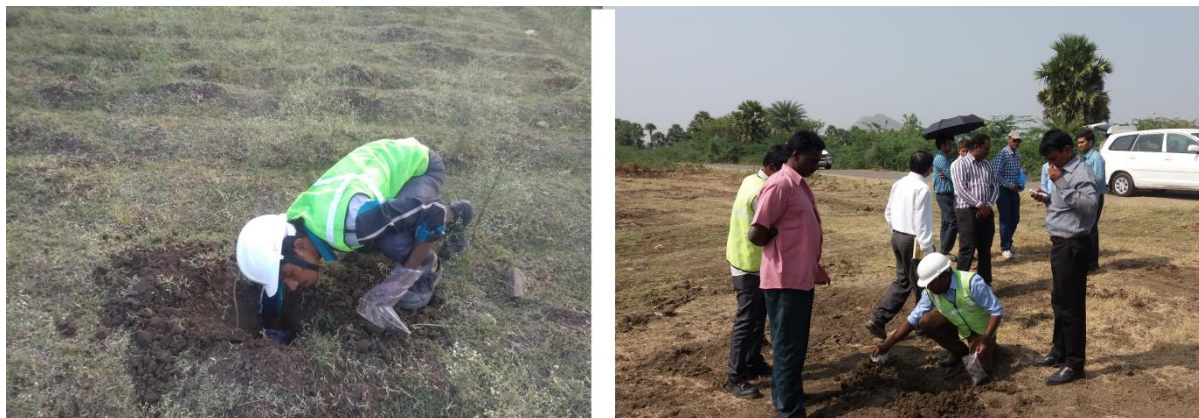
Figure 0-132 Soil sampling near Sakhamuru and Nekkallu using Crowbar
