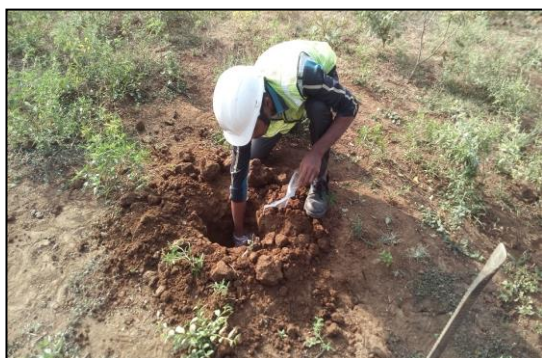
Figure 6-137: Soil sampling near Nidamaruru and Penumaka using Crowbar
