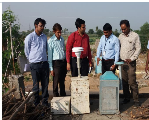
Figure 6-7 AAQ Monitoring stations installed at Malkapuram and Velgapudi
