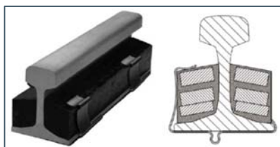
Figure 6-5_Typical tuned rail dampers cross section
