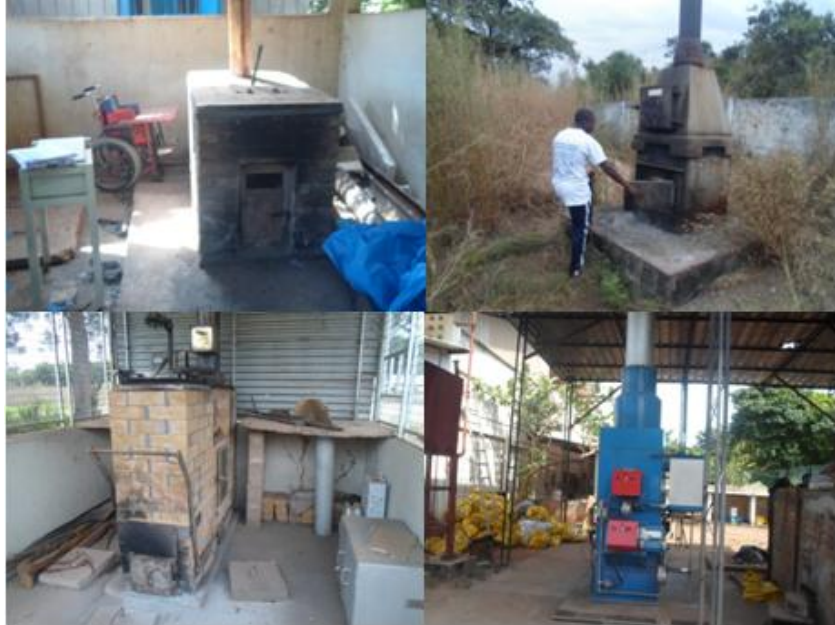
Figure 61 Various types of incinerators
