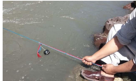
Sonar attached to graduated rope
