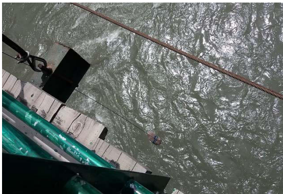
Verification of depths by using a rock and plumb line
