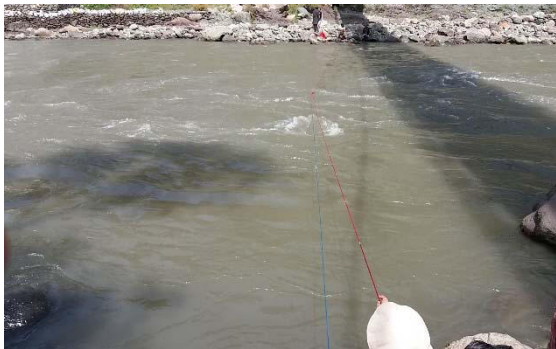
Cross section measurement at EF site 1-1
