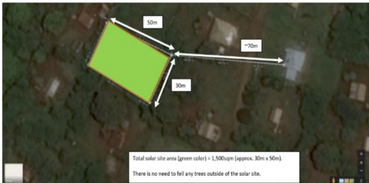
Figure 1 - The proposed Nomuka solar site and existing power station
