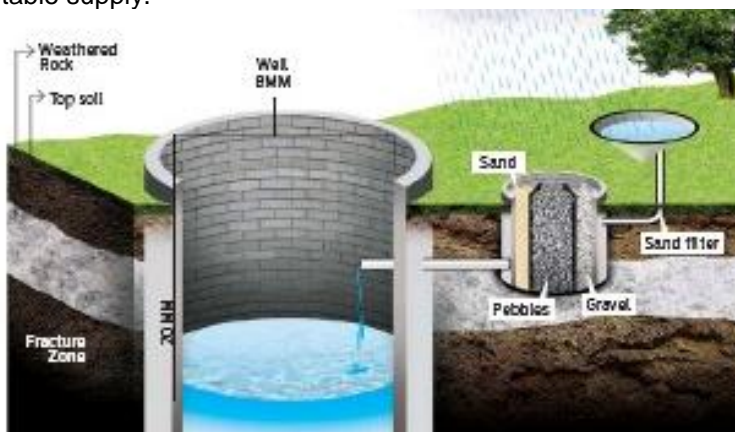
Induced recharge structure, Dharmapuri district, Tamil Nadu
