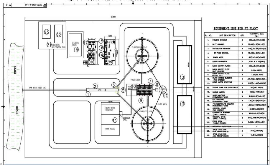
Figure 6: Layout Diagram of Proposed Water Treatment Plan
