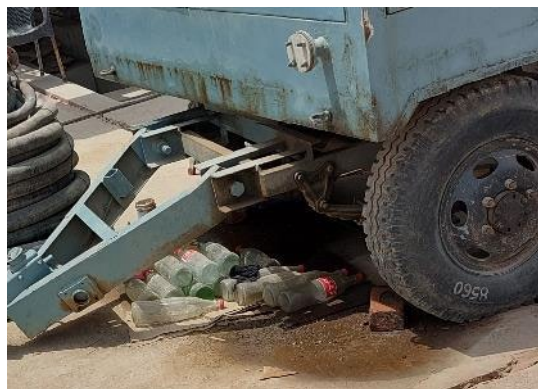
Fuel Oil Spill near a Diesel Generator under Use of Contractor
