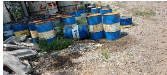
Unmarked Empty Drums of Transformer Oil on Unpaved Surface
