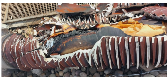
Burnt Circuit Breaker near the Affected Site
