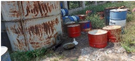
Empty Drums of Transformer Oil on Unpaved Surface. Residual Oil can be Seen in a Bowl
