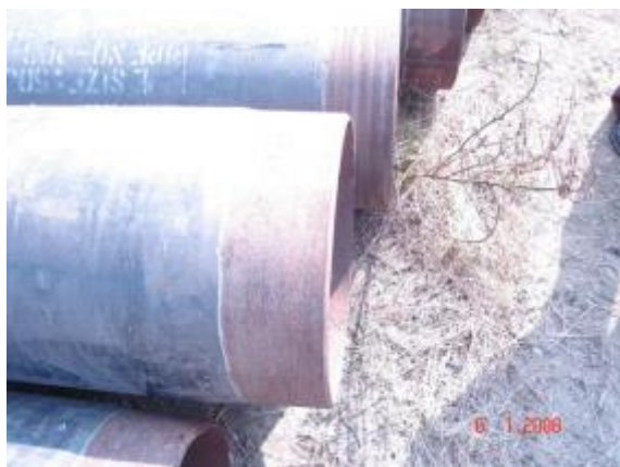
(a) 3-layer polyethylene (LPE) coating
