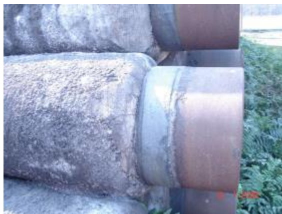
(b) Concrete weight coating
