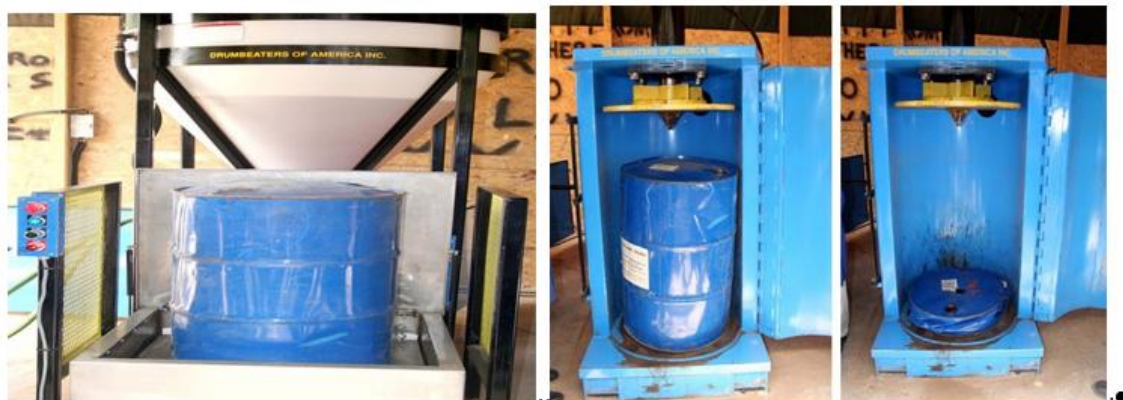
Figure 8: Automated solvent washing and crushing equipment ¶¶
