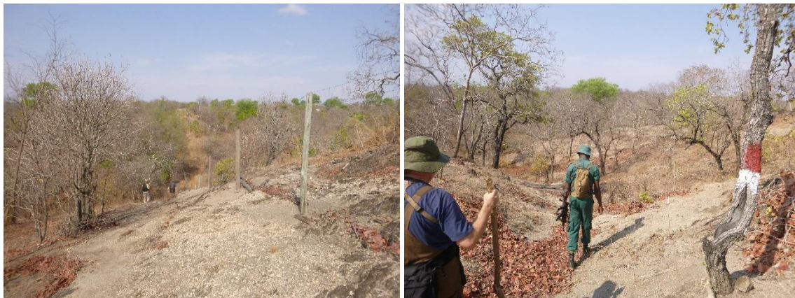
A topographic peg is visible on the tree on the right photo. Source: BRLi, 2016
