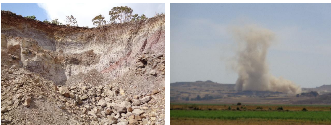
Figure 63 Borrow pit with dangerous steep slopes (left) and typical impact from blasting (right)
