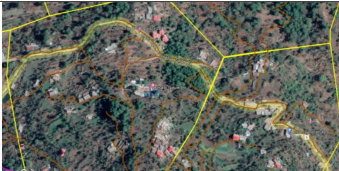
SS9: Proposed Rising Main on State Highway 9 from From Source T/Well at Barotiwal To SR Damuwala-2, (50 mm)
