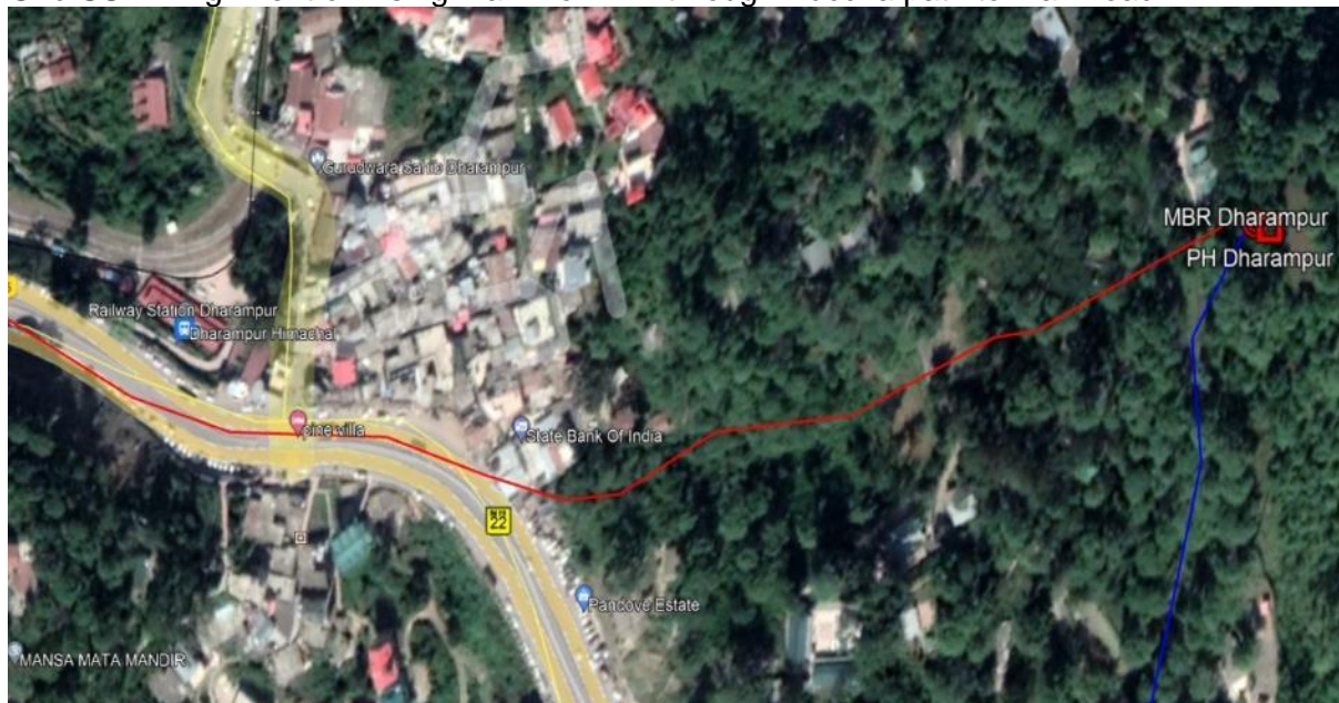
Grid SS-1: Alignment of Rising main from PH through Kuccha path to Main road.
