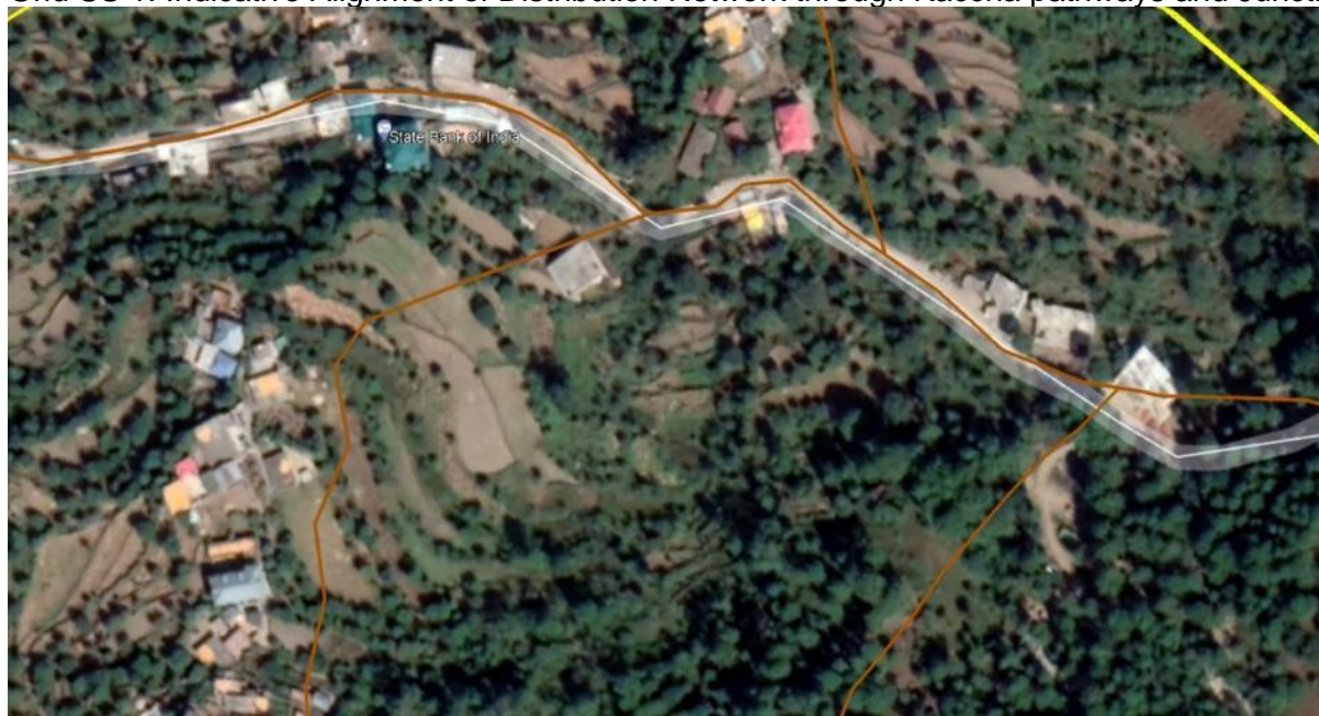
Grid SS 1: Alignment of Gravity Main from Source along with forest trails/ water stream
