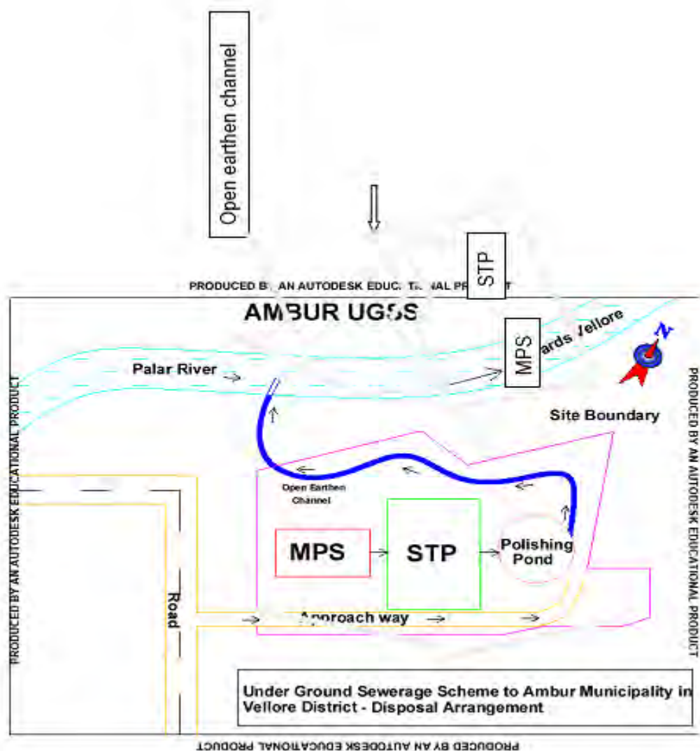
Figure 4: Sewage Treatment Plant and Alignment of Outfall open earthen channel
