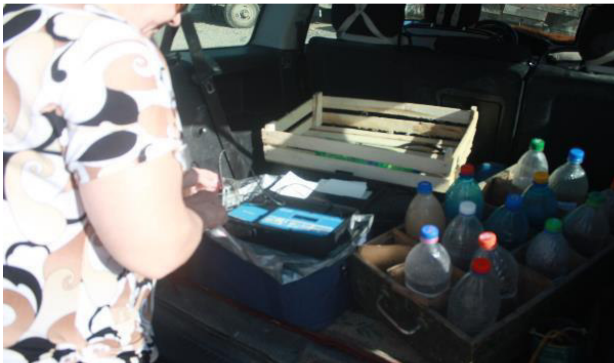
Pic 3. Conductivity meter for determination of salinity level and water electrical conductivity in Vakhsh River at Kyzyl-Kala Bridge
