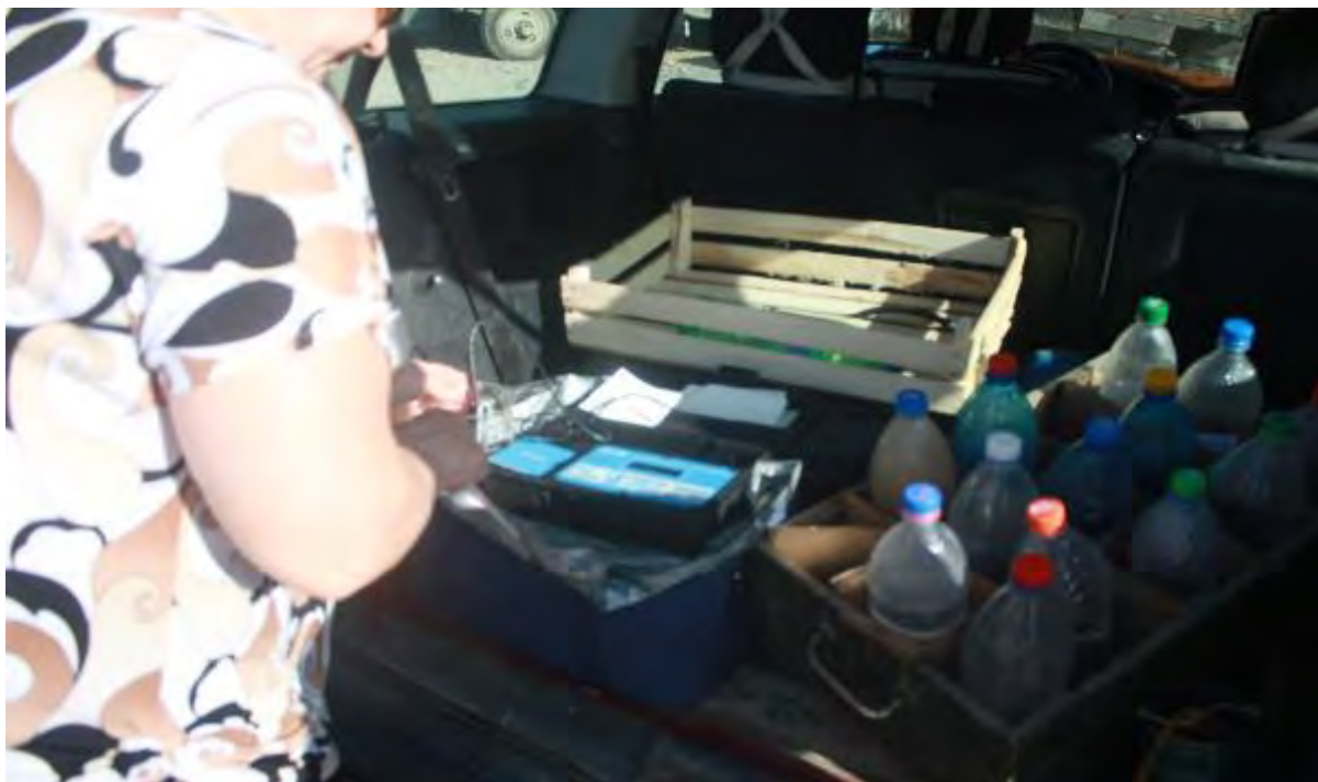
Pic 3. Conductivity meter for determination of salinity level and water electrical conductivity in Vakhsh River at Kyzyl-Kala Bridge
