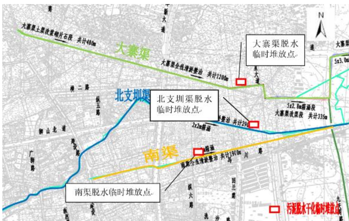
Figure 5-2 Fengxin county sludge dewater temporary storage site
