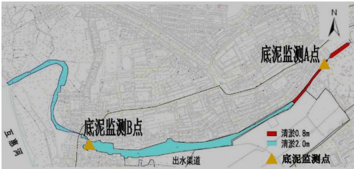
Figure 3-24 Sediments Monitoring Points Map of the Outlet Canal of Pipa Lake in Yugan County
