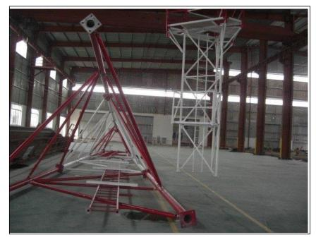
**Photo 1:** Prefabrication Tower Segements at Steel Factory
