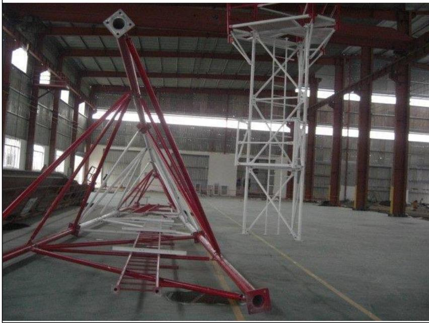
**Photo 1:** Prefabrication Tower Segements at Steel Factory
