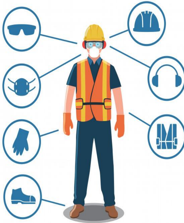
Figure 11: PPEs required in construction, operation, and maintenance activities of roads
