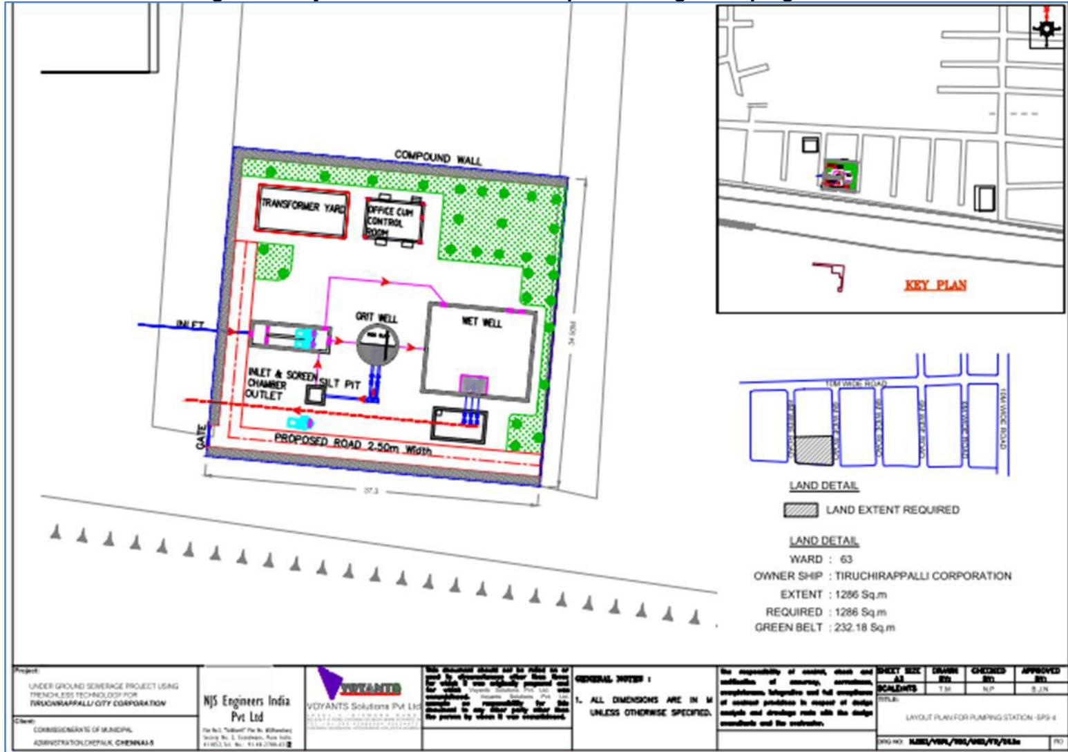
Figure 5: Layout Plan on Revenue Map for Sewage Pumping Station 6
