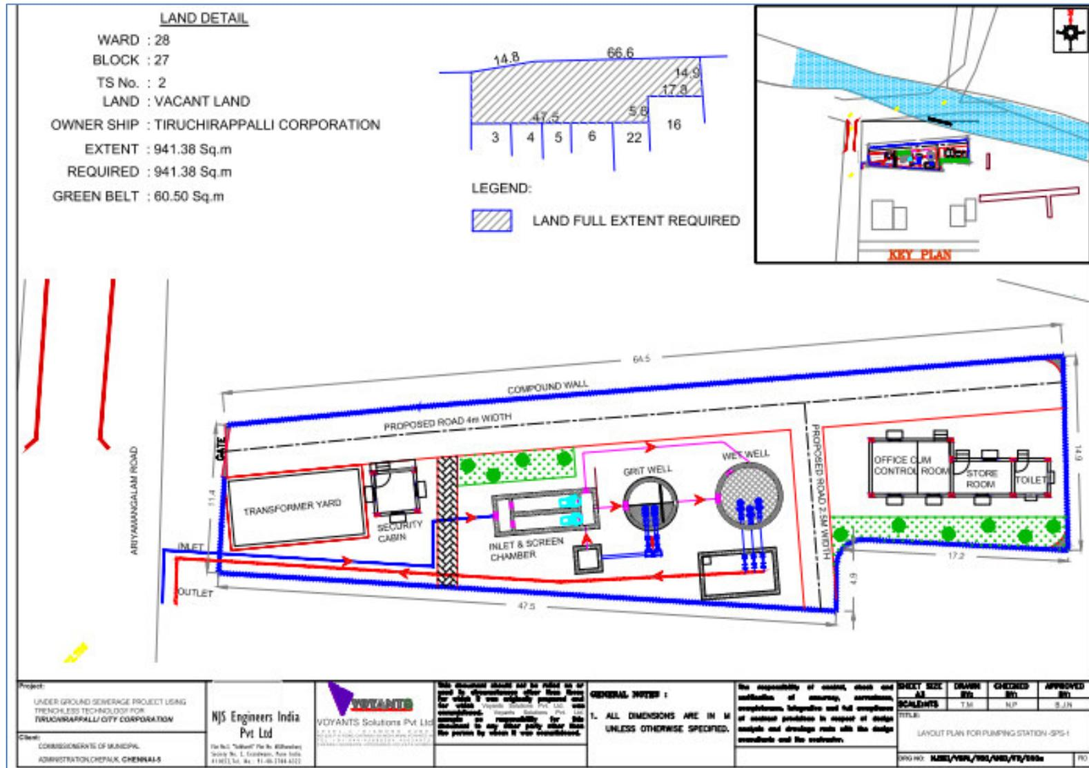
Figure 2: Layout Plan on Revenue Map for Sewage Pumping Station 2
