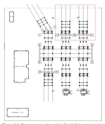
Figure 3-2: Planned extension of the Doshi Substation (red square)
